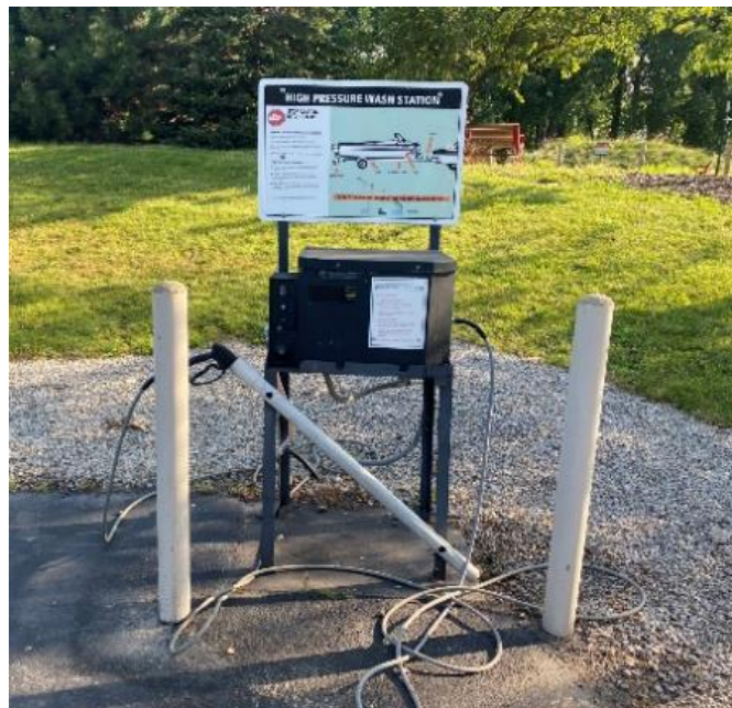
Figure 6-5. High pressure wash station available at the Fritse Park Boat Launch.
