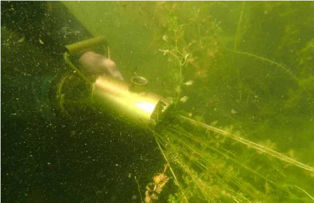
Figure 8-4. DASH diver feeding plants into suction device.
