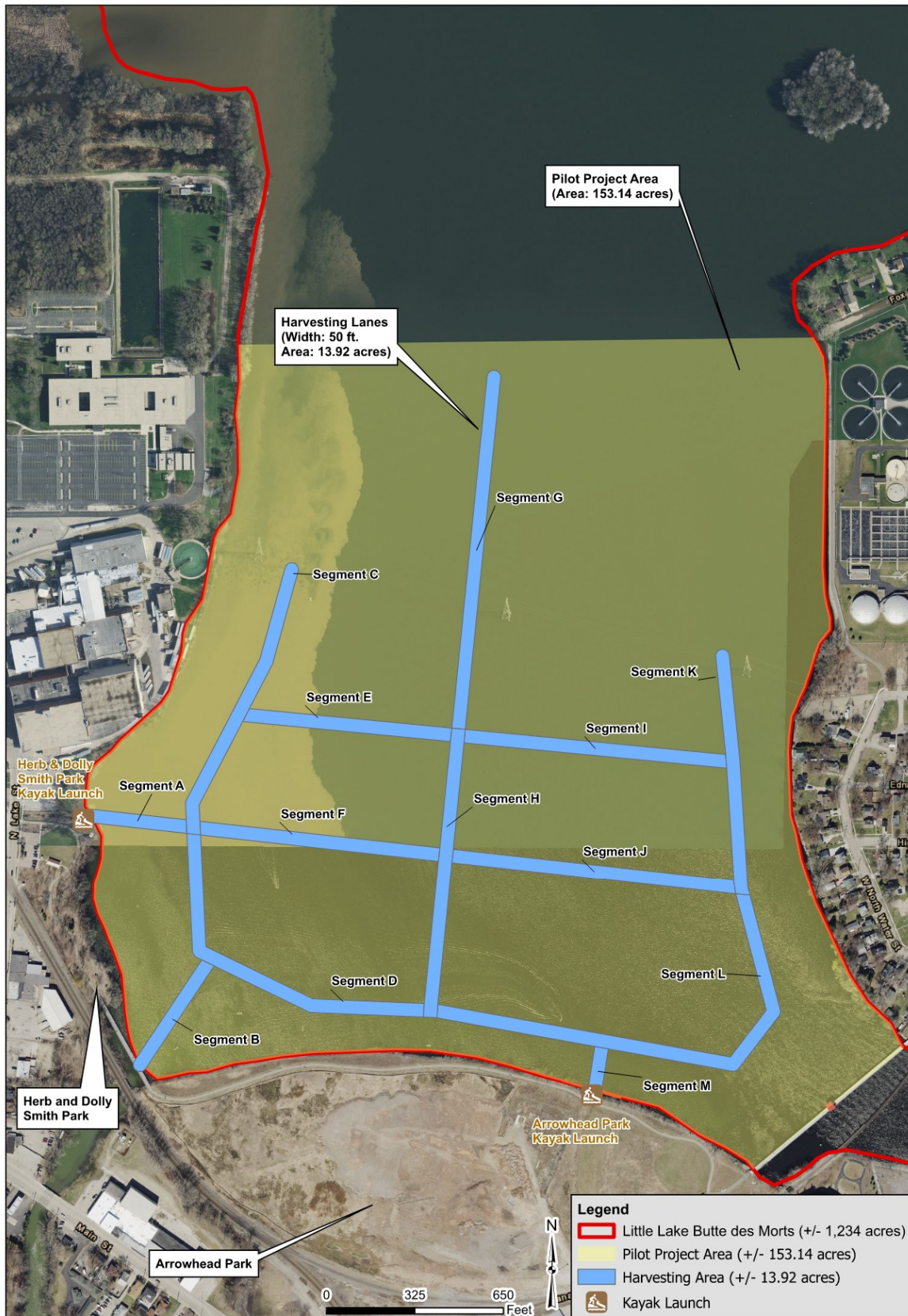
Figure 8-1. Harvesting lanes and segments within Pilot Project Area.
